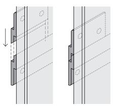
10 Slide Panel down to engage Wall and Panel Z-Clips
